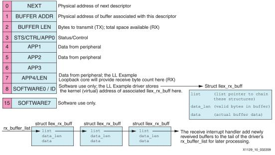
Figure 10: DMA Receive Descriptor Usage
