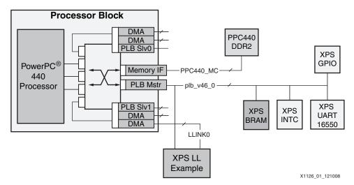
Figure 1: Reference System Block Diagram
