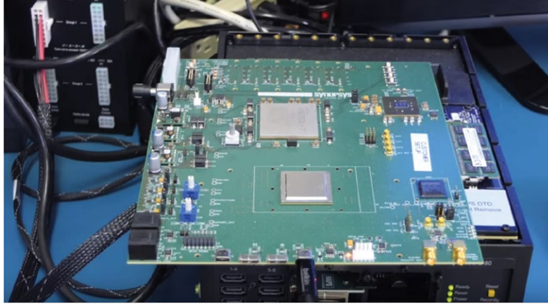
Figure 5: Synopsys HAPS-80 FPGA-based prototyping system used to develop and test USB 3.2 IP
