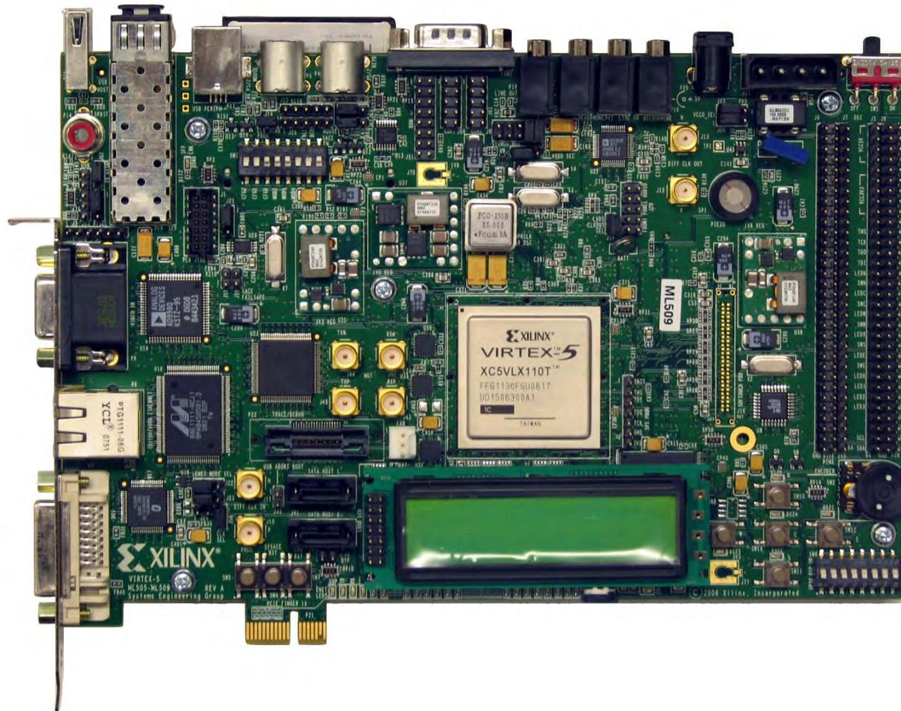
Note: The XUPV5-LX110T uses an XC5VLX110T FPGA.
